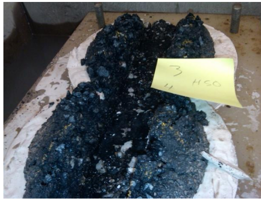
Figure 15: Completed Limestone ERSA Specimens
